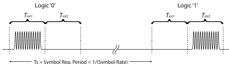
Fig. 24 Pulse position modulation represents data by the presence of a pulse in a particular window in time
