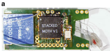
Fig. 13 Flexible PCB (a) top and (b) side
