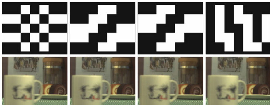
Fig. 11 Four multiplexing aperture codings and the corresponding captured images. Upper row shows four of the 31 aperture patterns that we generate from an S-Matrix. Bottom row shows the four corresponding captured images
