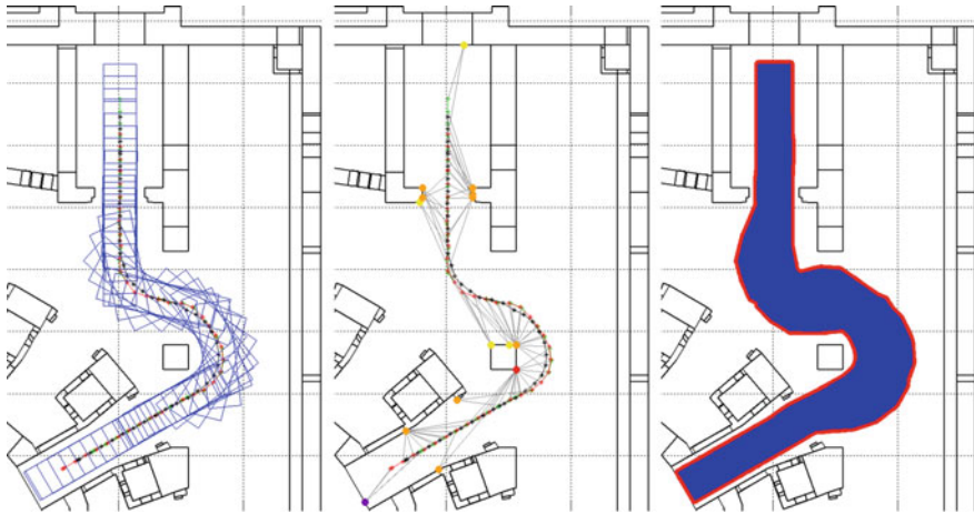
Fig. 26 Trajectory to port 2 in level B1 of TB using line guidance (from left to right): path and sampling poses, the most closest obstacles and the area spanned by the vehicle along the path, with a safety margin
