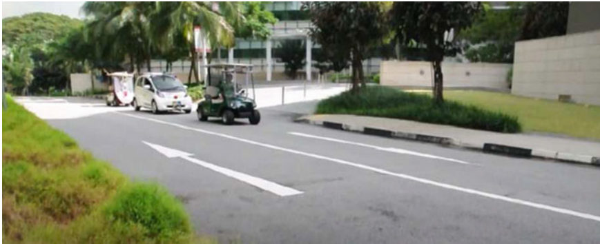
Fig. 1 Our autonomous personal transporters in operation, providing Mobility-on-Demand service in a campus environment of National University of Singapore
