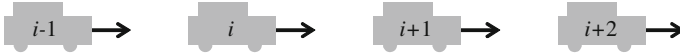
Fig. 8 Concept of leader string where i is an ego vehicle. i + 1 and i + 2 are the first and second leader of i , respectively. i - 1 is a following vehicle behind ego vehicle i
