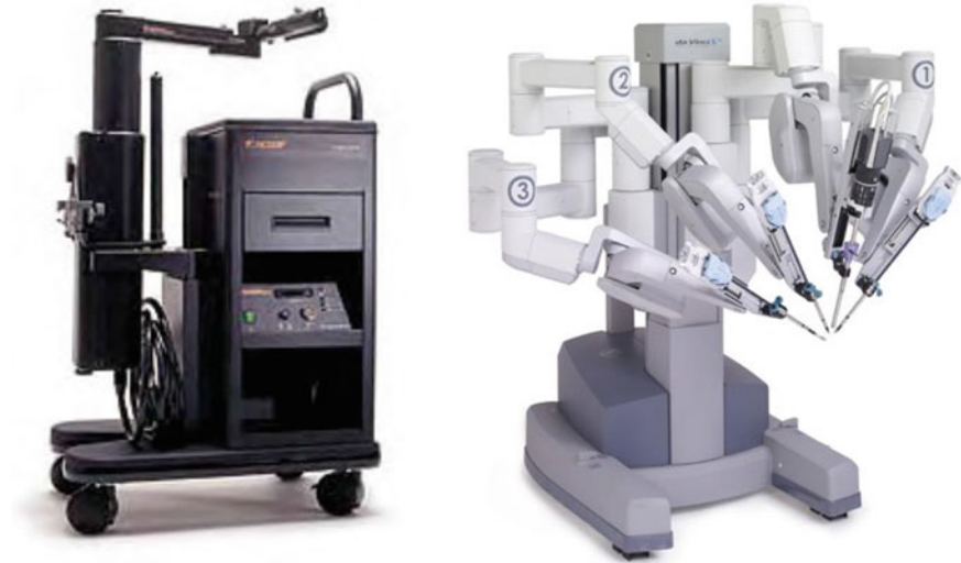
Fig. 3 The AESOP robot laparoscopic assistant on the left and the Da Vinci system on the right
