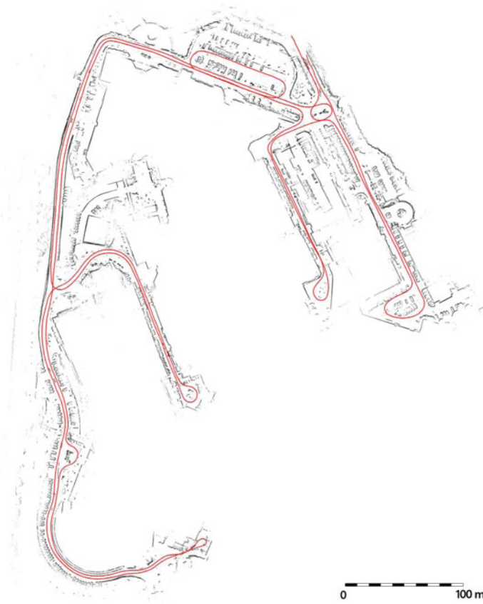
Fig. 6 Localization result of AMCL within NUS Engineering Campus
