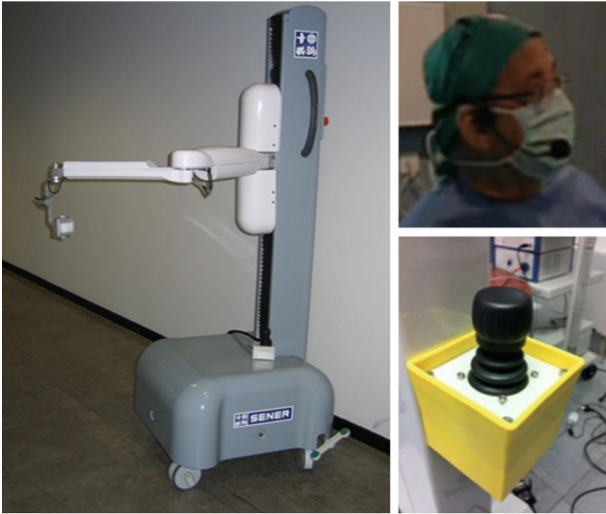
Fig. 13 ERM system for holding the laparoscopic camera ( left ) and its user interface based on the surgeon's voice or joystick device ( right )
