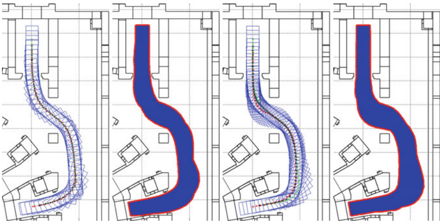
Fig. 31 Trajectory to port 1 in level B1 of TB ( from left to right ): line guidance and the corresponding spanned area, free roaming and the corresponding spanned area
