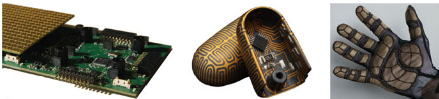
Fig. 3 Recent tactile sensors from Bielefeld University. From left to right a modular, flat 16 \times 16 tactile sensor array, a 3D shaped tactile fingertip suitable for the Shadow Robot Hand, and a flexible tactile glove manufactured from conductive fabrics
