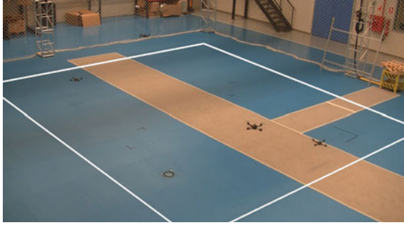
Fig. 18 Snapshot from the experiment where 4 quad-rotors implement an area partitioning strategy from a distributed manner using an algorithm based on the one-to-one coordination. The white solid lines defines the area to monitor
