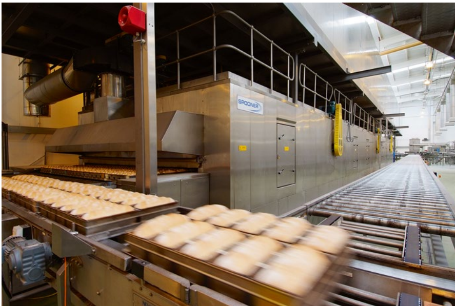
Fig. 5.11 Four-piece pan loaves entering the oven (courtesy Spooner Industries)
