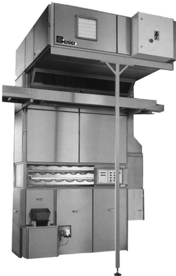
Fig. 4.14 Pocket type first prover (courtesy Benier)
