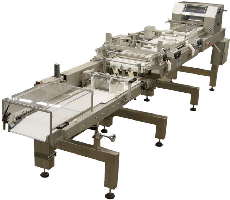
Fig. 4.22 Typical bread dough moulder for four-piece bread (courtesy Benier bv)
