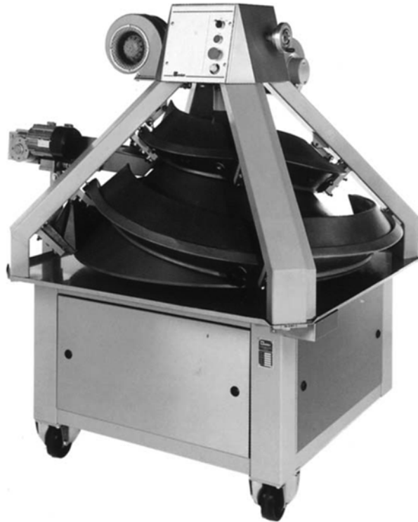
Fig. 4.12 Typical conical rounder, note this model has operator adjustable tracks (courtesy Benier bv)
