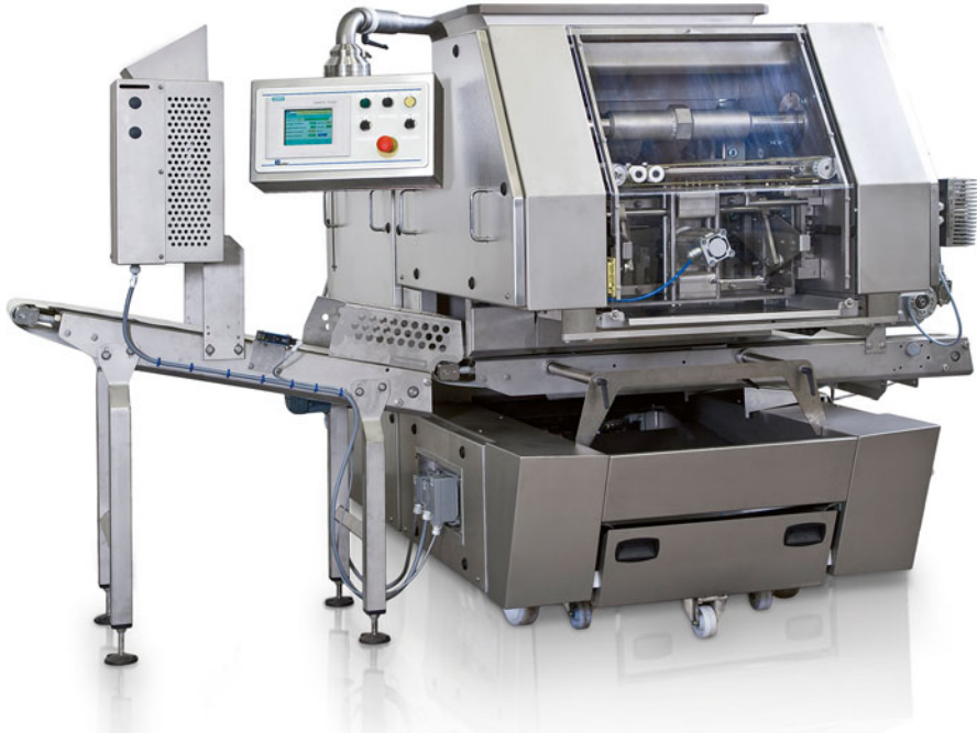
Fig. 4.9 Multi-pocket bread dough divider (courtesy Benier bv)
