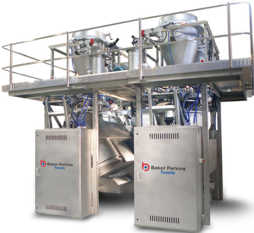
Fig. 4.2 Mixer and ingredient feed system for CBP doughs (courtesy Baker Perkins)
