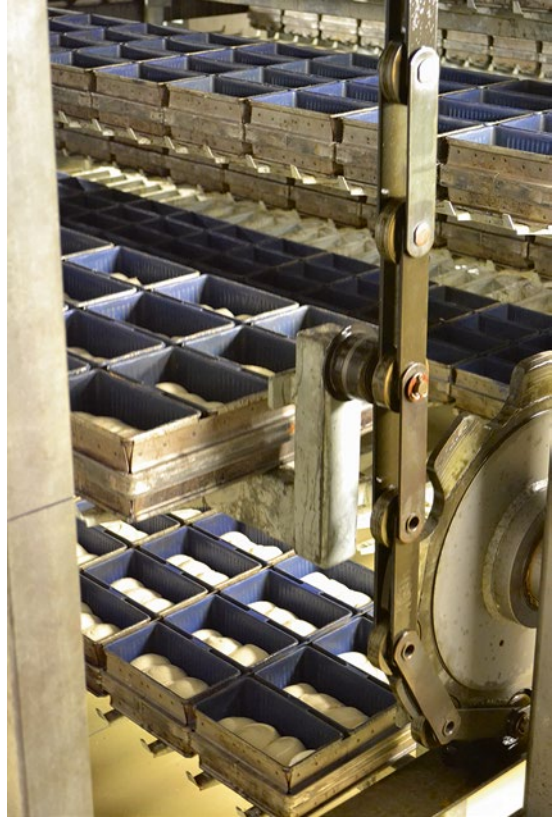
Fig. 5.8 Four-piece pan bread in the prover (courtesy Spooner Industries)
