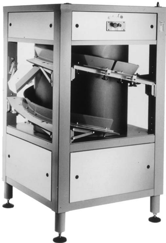
Fig. 4.13 Typical vertical drum rounder (courtesy Benier bv)
