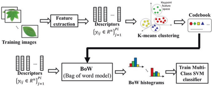
Fig. 7 An illustrated example of the learning stage in the proposed BoW-based leaf image recognition framework
