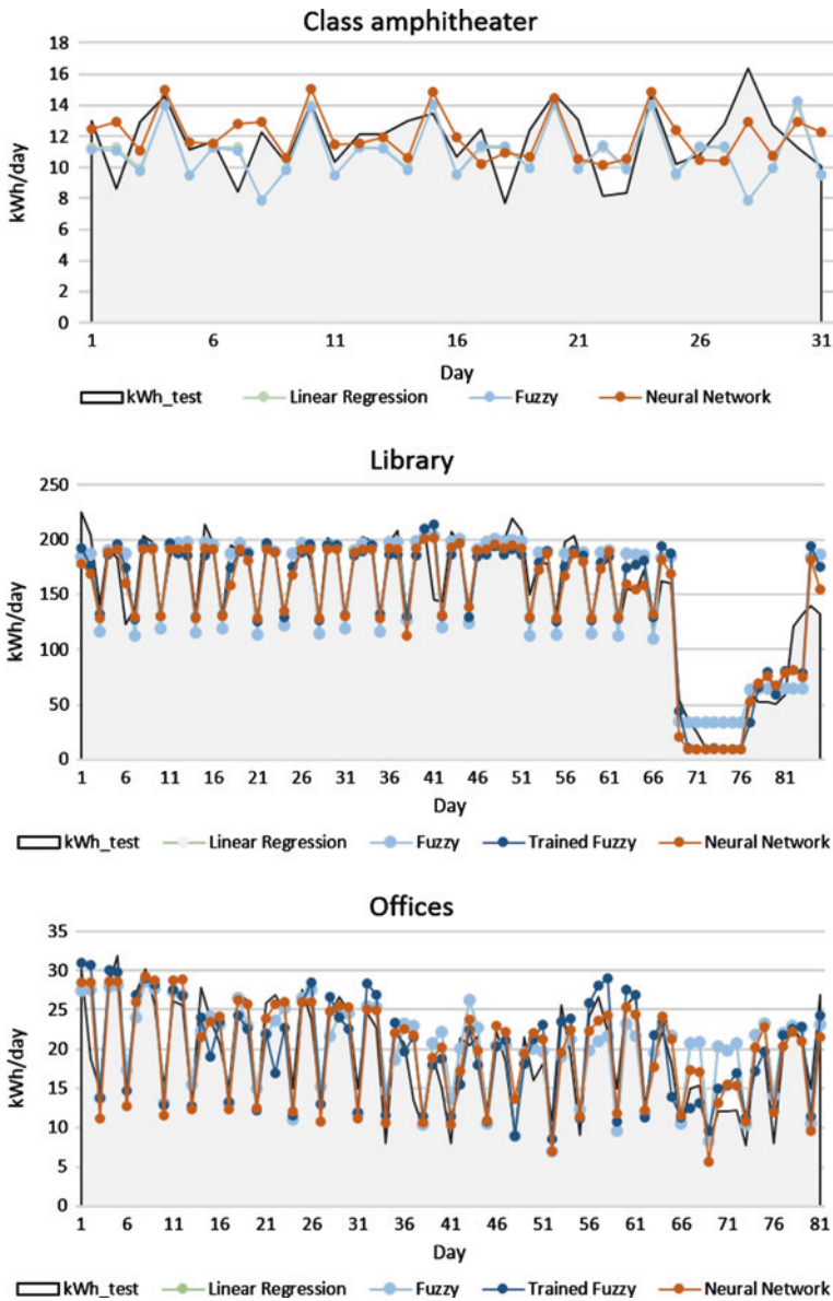
Fig. 2 Graphical representation of the modeled and the real electricity consumption for the three experimental spaces, concerning all models
