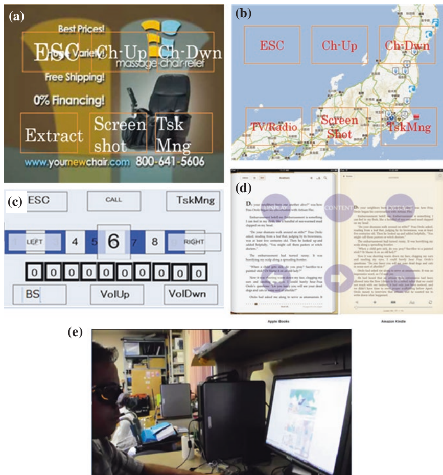
Fig. 16 Information collection aid with the proposed EBHCI. a Watching TV. b Listening radio. c Phoning. d Reading e-book. e Outlook of the information collection aid system (reading e-comic)
