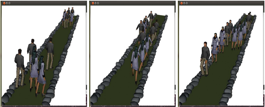
Fig. 6. Stills of three moments of a simulation with virtual pedestrians using data from the TS-ALL case of study. The agents are initially placed in random positions on the sides of the corridor.
