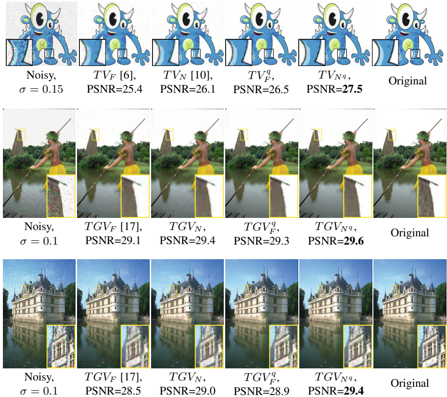
Fig. 5. Denoising of a piecewise constant image and natural images with TV^q ( q = 0.5 ) and TGV^q regularization ( q = 0.75 ) using the proposed primal-dual algorithm. We chose \alpha = 1/3 for all the TGV experiments and the data fidelity parameters were optimized for maximal PSNR.
