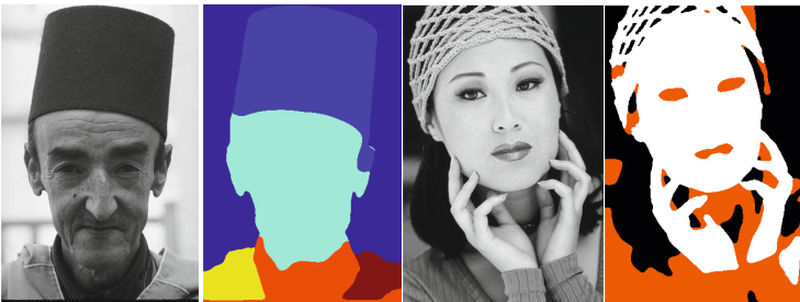
Fig. 3. Supervised example segmentation of two natural images from the Berkeley database with 6 and 3 regions, respectively. The contours are initialized via seeds placed by a user and convergence achieved if less than 50 pixels change between iterations. From left to right: Image and corresponding segmentation.
