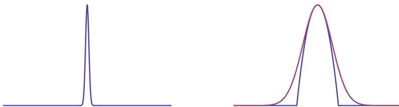
Fig. 3. Using the function e^{-\frac{x^2}{2\epsilon^2}} to approximate indicator function (Left) by \epsilon = 0.005 and (robust) truncated quadratic loss (Right) by \epsilon = 1/2 . Both cases are plotted in the range x \in [-4, 4] .
