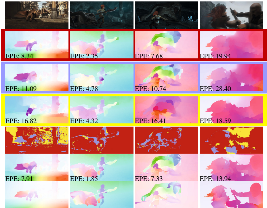
Fig. 5. Examples of our multi-frame fusion from the MPI-Sintel Final training set. Top row: Frame at time t . Rows 2-4: Inertial estimates of the flow [t \rightarrow t + 1] , -[t \rightarrow t - 1] , and \frac{1}{2}[t \rightarrow t + 2] . Row 5: Fusion classification for each pixel. Color indicates the estimate used at each pixel. Colors correspond to the border colors of the inertial estimates. Row 6: Fused flow estimate. Bottom row: Groundtruth flow. For all flow estimates, the endpoint error is printed in the image.
