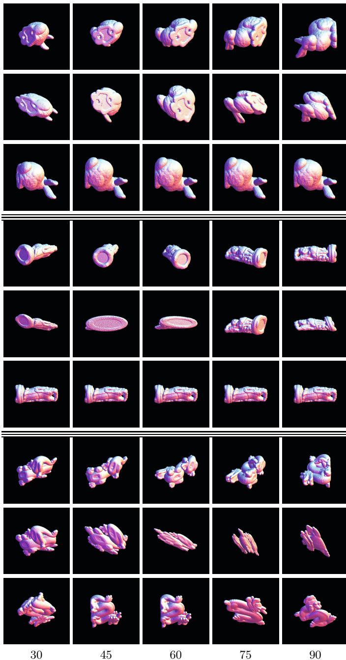
Fig. 2. Each object occupies three successive rows, where each row has the following role. (Top) Input \mathcal{P} , which is a rotated version of \mathcal{Q} . (Middle) Transformed \mathcal{P} to match \mathcal{Q} using ICP. (Bottom) Transformed \mathcal{P} to match \mathcal{Q} using proposed method.
