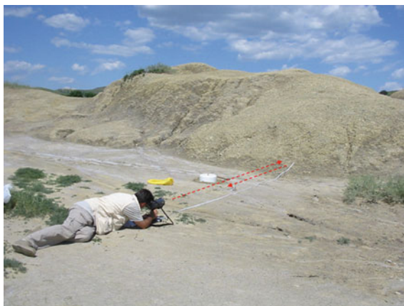
Fig. 4.3 Detection of anomalous concentrations of methane in the air a few centimetres above the ground using a portable laser sensor (Fierbatori seepage area, Berca oil-field, Romania; photo by C. Baciu)
