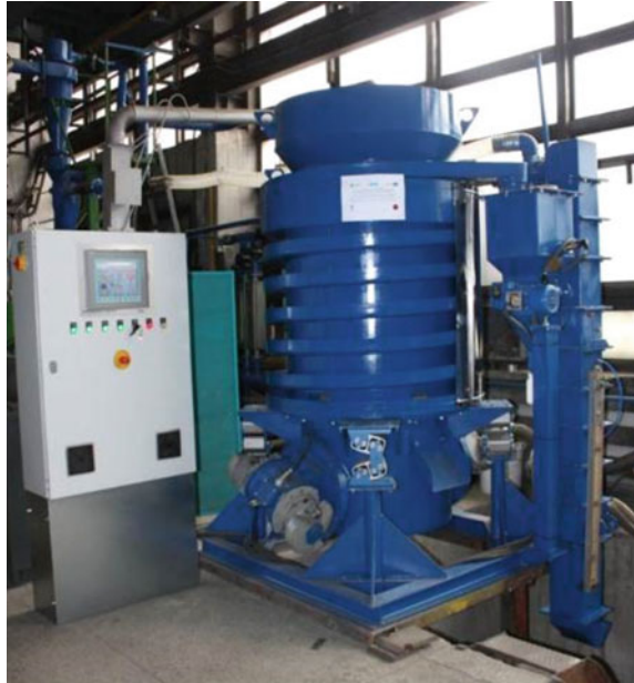
Fig. 4.8 View of REGMAS 1.5 reclaimer at the testing site at Faculty of Foundry Engineering AGH University of Science and Technology, Poland
