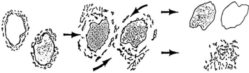
Fig. 4.4 Pictorial diagram of liberating sand grains from coatings of spent binding material—as a result of the elementary rubbing operation [1]
