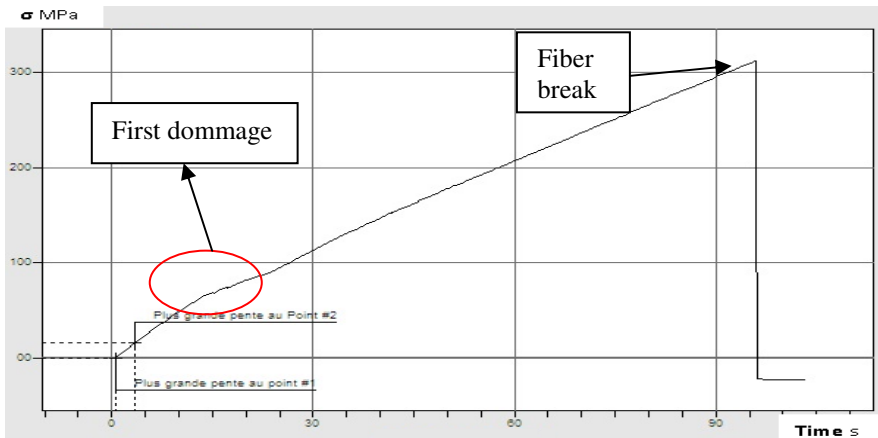
Fig. 7 Stress-Time curve for a composite plate with hole ( a=4\text{mm} )
