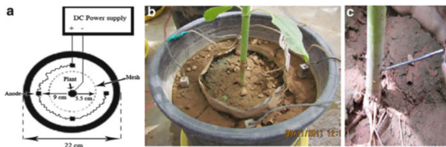
Fig. 20.9 (a) Diagram of the soil remediation system, (b) graphite electrodes placed around the pots as anodes, (c) stainless steel needle inserted in the lowest part of sunflower stem for charging the plant with negative charge (Adopted from Tahmasbian and Safari Sinegani 2014)
