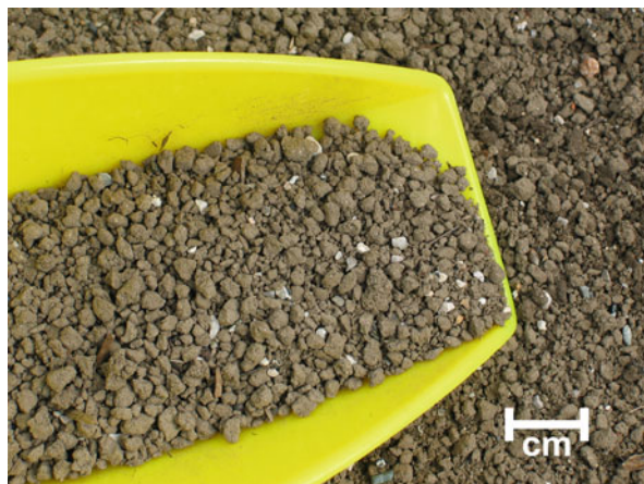
Fig. 21.4 Artificial aggregates of remediated soil formed by rubbing soil through 5 mm mesh sieve
