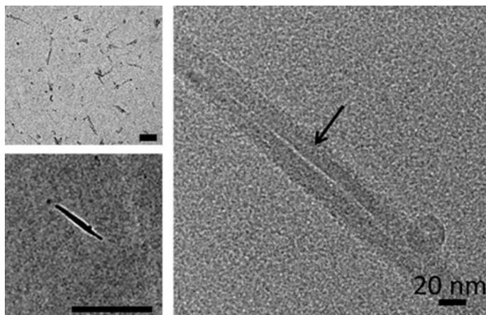
**Fig. 10.1** Transmission electron micrograph of single-walled and multi-walled carbon nanotubes. *Top left* Single-walled carbon nanotubes. *Scale bar* 100 nm. *Bottom left* Multi-walled carbon nanotubes. *Scale bar* 500 nm. *Right* Zoomed image of multi-walled carbon nanotubes. The *arrow* indicates the thick wall of the nanotubes. Reprinted and adapted with permission from (Serag et al. 2011a, b). Copyright (2011) American Chemical Society
