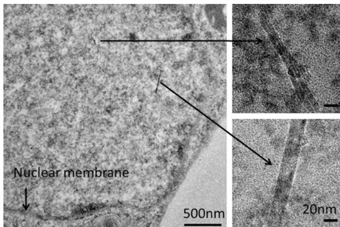
**Fig. 10.6** Transmission electron micrographs showing carbon nanotubes accumulation inside the nucleus of *C. roseus*. *Left* The micrograph shows multi-walled carbon nanotubes inside the nuclear matrix. *Right* The corresponding zoomed-in images of the nucleus. Reprinted and adapted with permission from (Serag et al. 2011b). Copyright (2011) American Chemical Society
