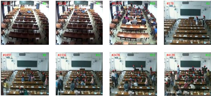
**Fig. 7.** Counting result in *video1* and *video2*, the number of human was marked in green on the top right corner of images, and the clustering result was marked on the head of human in red points.
