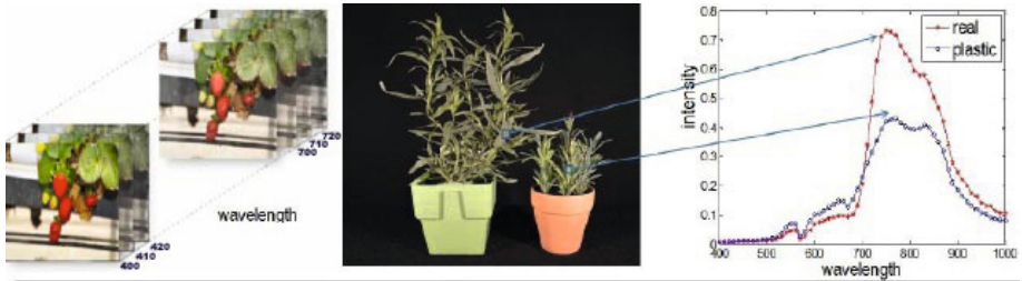
Fig. 1. A hyperspectral image (left) with different slices correspond to wavelength and an example of intensities (right) for real and plastic objects in different wavelengths
