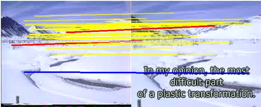
Fig. 2. An example of filtering false matching pairs. Left: a key frame extracted from an indexing video; Right: a key frame extracted from a query video with transformations of resizing and subtitles. All the lines denote matching pairs of original SURF descriptors. Red lines denote the false matching pairs which are filtered by adaptive LSH using bucket splitting; Blue lines denote the false matching pairs which are filtered by Descriptor Filtering method based on relative distances; Yellow lines denote the right matching pairs which compose the candidate sets after pruning in our algorithm.
