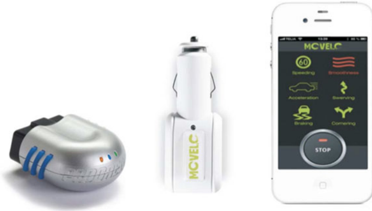
Fig. 1 Progressive insurance snapshot measurement probe for the on-board diagnostics ( left ); sensing device for the cigarette lighter outlet by Movelo ( middle ); and smartphone with insurance telematics software from Movelo ( right )
