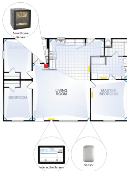
Fig. 2. Floor plan of a VA SmartHome including examples of interactive panels and sensors.
