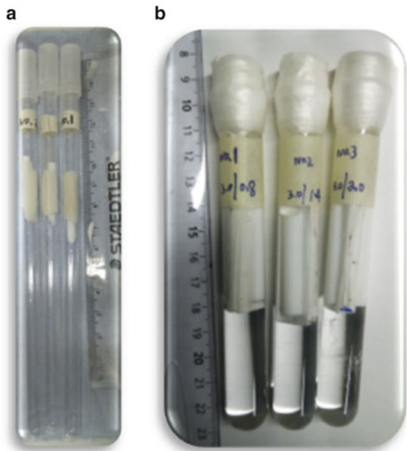
Fig. 12.13 (a) Fibre bundle-based MR phantom; (b) Fibre strip-based MR phantom
