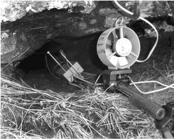
Fig. 22.12 An ultrasonic anemometer (left) and a mechanical anemometer (right) recording data are located in the bat access hole to measure the rate of air flow (photo by P. C. Lucas)
