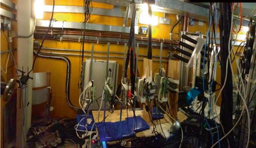
Fig. 1.5 Neutron experiment Setup in ISIS for FPGAs and GPUs
