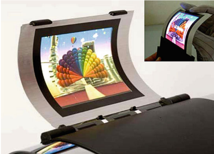
Fig. 18 Photographs of a 4-in. flexible AMOLED panel fabricated using low-temperature a-Si TFT backplane on a stainless steel substrate, under inward and outward bending (Ma et al. 2010)
