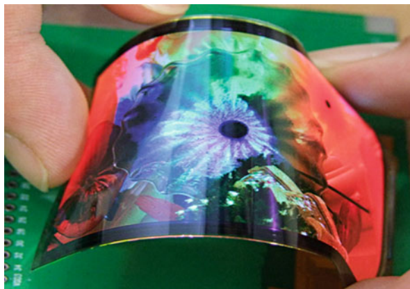
Fig. 22 Photograph of a flexible 2.8" QVGA AM OLED fabricated by the in situ plastic coating method involving a plastic film with a CTE of 3 ppm/K and process temperature capability of 350 °C, and LTPS TFTs (An et al. 2010)
