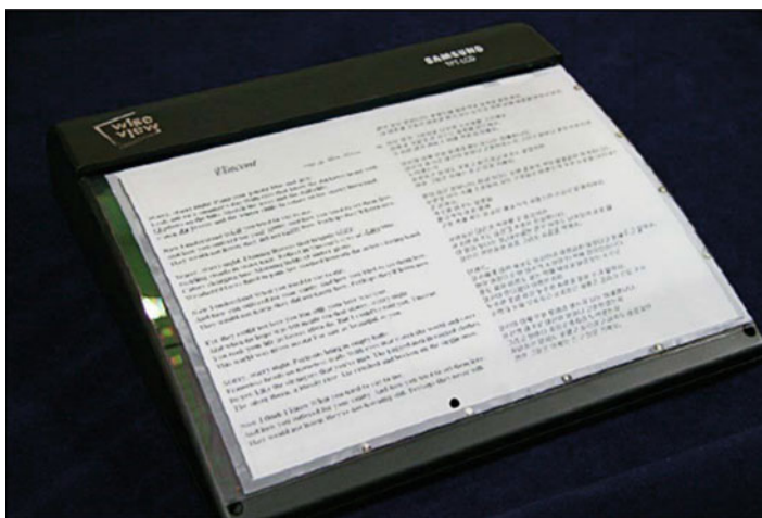
Fig. 17 Photograph of an AM EPD display fabricated using low-temperature a-Si TFTs backplane on a flexible PEN plastic backplane (Hwang et al. 2007)
