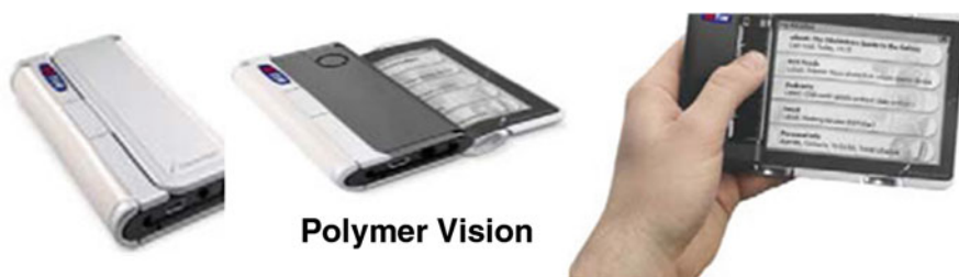
Fig. 3 Example of a foldable electrophoretic display by Polymer Vision (Kato et al. 2010)
