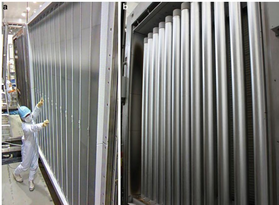
**Fig. 2** Large-size (G8/8.5) sputtering systems provided by (a) ULVAC (Matsuda et al. 2013) and (b) AKT (Kloepfel et al. 2013) for IGZO sputtering
