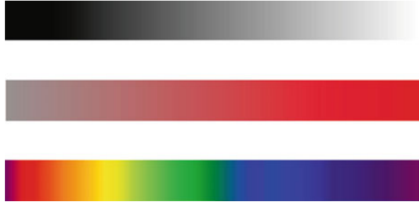
Fig. 1 The three attributes of color vision: lightness ( upper ), chroma ( middle ), and hue ( lower )
