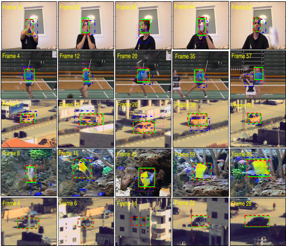
Fig. 4. Visual examples of LFR tracking for 3 and 5 frames per second videos with target objects marked by: ground truth - dashed line ; The proposed method - regular line ; KLT - dotted line ; particle filter - dashed-dotted line. The first four examples compare all the methods in different time frames. In the last example we compared our method to the ground truth.
