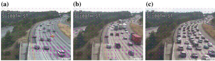
Fig. 13.4 Illustration of the Farneback dense optical flow vectors for sample video frames of different traffic congestion levels in the UCSD dataset— a light traffic b medium traffic c and heavy traffic
