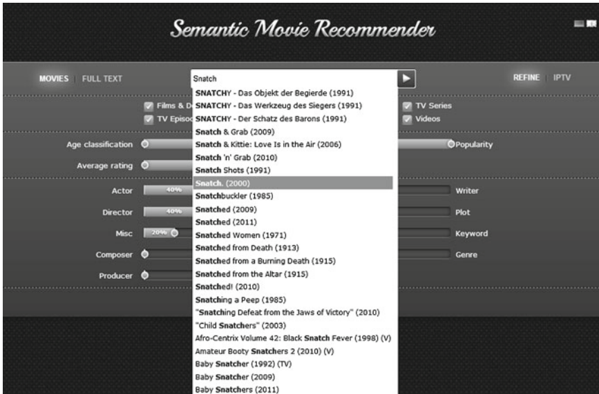
Fig. 5.5 The figure shows the auto-completion function suggesting the user entities matching the user string input. This avoids problems with ambiguous queries and allows the system to compute recommendations directly on the semantic graph
