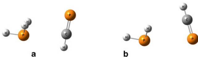
Fig. 8.34 H_3P:PCH complexes with conformations B and C. Complexes have C_s symmetry except for H_2(CN)P:PCCN and H_2(CCH)P:PCCCH B which have C_1 symmetry. (Reprinted with permission from Ref. [36]. Copyright (2014) Springer Science and Business Media)
