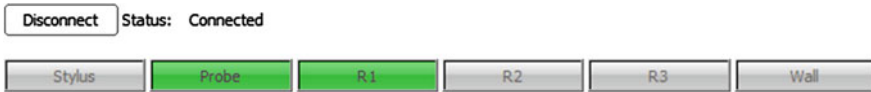
Fig. 3 The tool viewer shows the visibility of the markers. The spatial position of the US probe (Probe), three references markers (R1, R2 and R3) attached to the patient, a Stylus and a marker attached to the wall that faces the patient are acquired by the software. Currently, only the Probe, R1 and the Wall are used to compute the angle between the vertebrae but in the future we plan to explore the use of the others to improve the workflow
