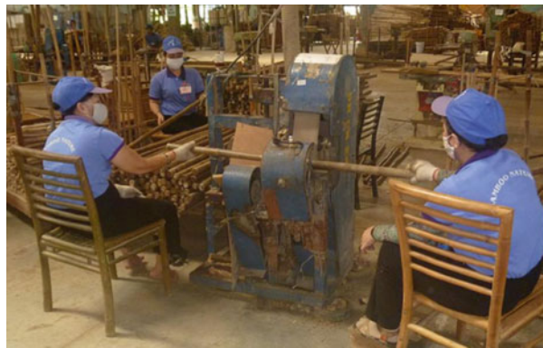
Fig. 9.26 Skin removal by sanding, Co. Bamboo Nature, South Vietnam (Tang and Liese 2011)
