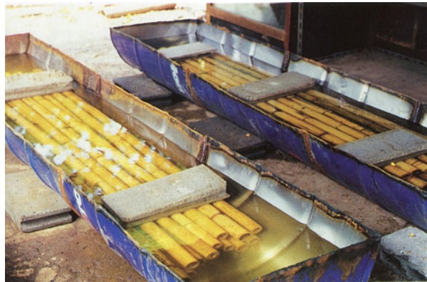
Fig. 9.25 Soaking method (Liese and Kumar 2003)
