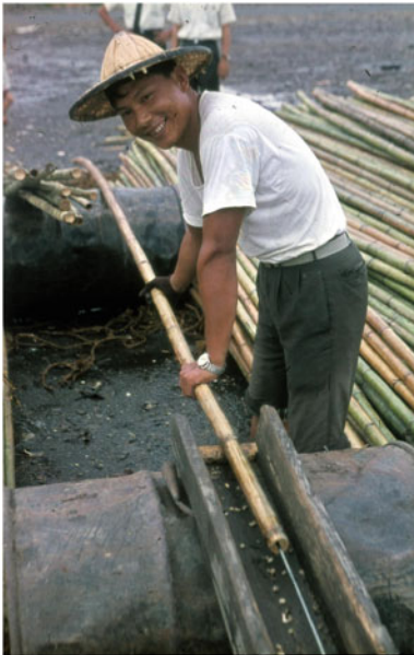
Fig. 9.31 Ruptured nodal walls by a long iron stick to ease penetration in Thailand (Liese and Kumar 2003)
