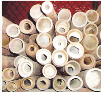
Fig. 9.31 Ruptured nodal walls by a long iron stick to ease penetration in Thailand (Liese and Kumar 2003)
