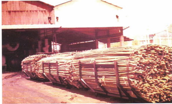
Fig. 9.30 Culms loaded for pressure treatment, Taiwan (Liese and Kumar 2003)
