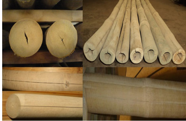
Fig. 9.35 Drying defects: end checks and splits (Tang et al. 2013)
