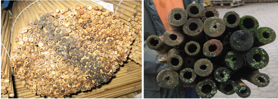
Fig. 9.4 Moulded bamboo culm parts at arrival in Hamburg after shipping from Vietnam (Tang 2013)
