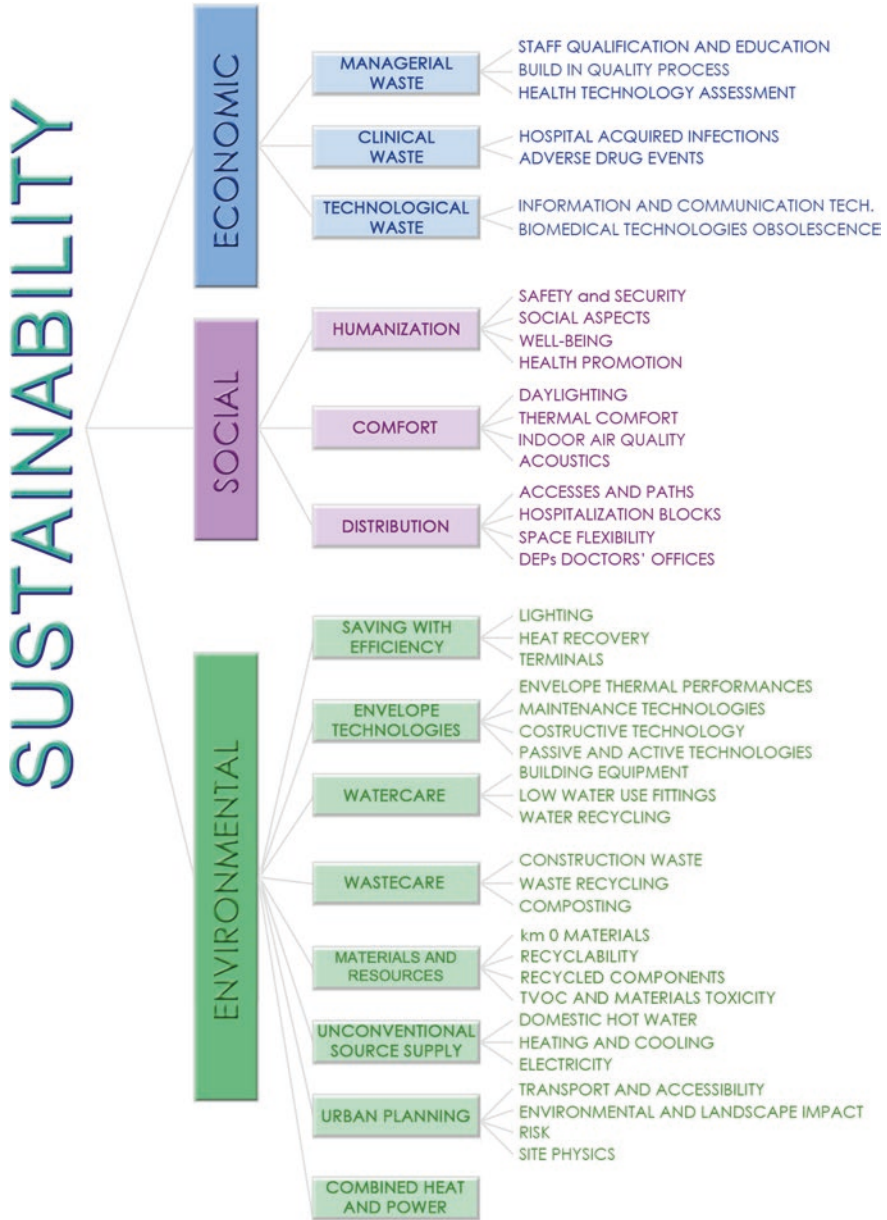
Fig. 4.3 Global SustHealth system for in-design hospital according to the structure of the macro-areas criteria and indicators
