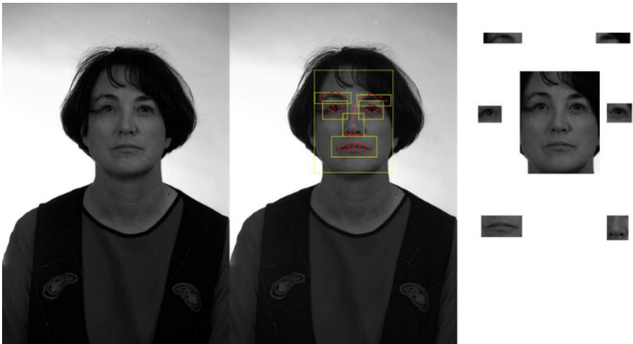
Fig. 4. (a) Face image of a women [18]. (b) ROI selected on the image. (c) ROI cropped.
