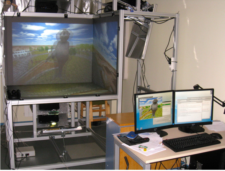
Fig. 1. The “Kyb3” Virtual Reality Environment, showing a 3D model in Blender-CAVE
