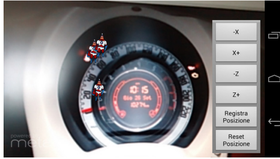
Fig. 4. Inserting of the positions of the light using training module
