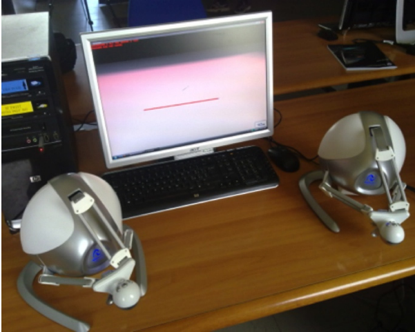
Fig. 5. The serious game using two Novint Falcon haptic devices
