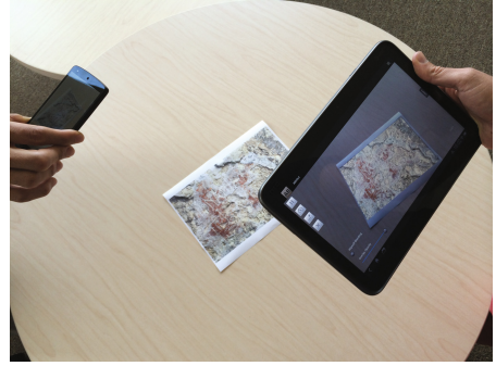
Fig. 6. Interactive RTI visualization using multiple collaborating mobile devices serving as viewer and virtual light source
