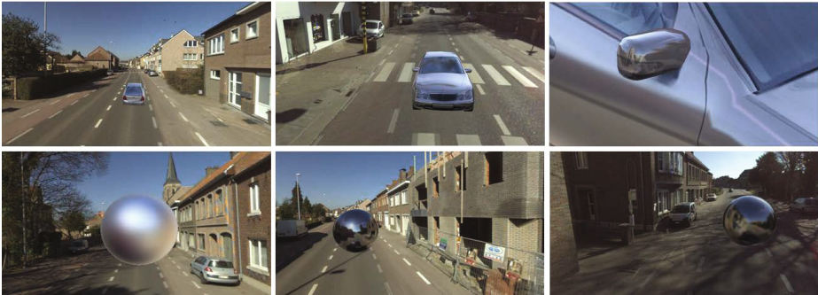
Fig. 1. Illustration of real-time augmented rendering of virtual objects in an omnidirectional environment. The 360° video is used as environment map for realistic lighting.
