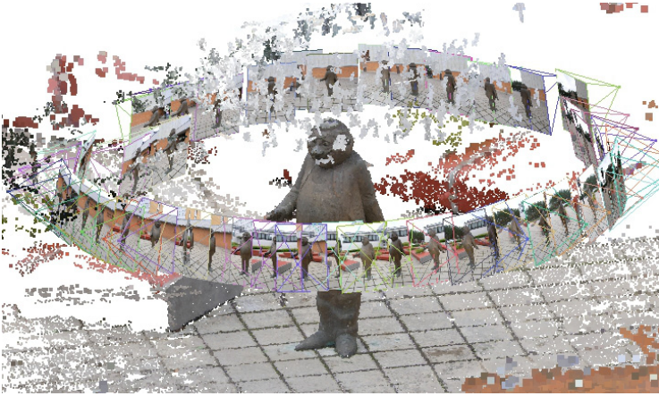
Fig. 7. Point cloud with camera positions obtained with VisualSFM
