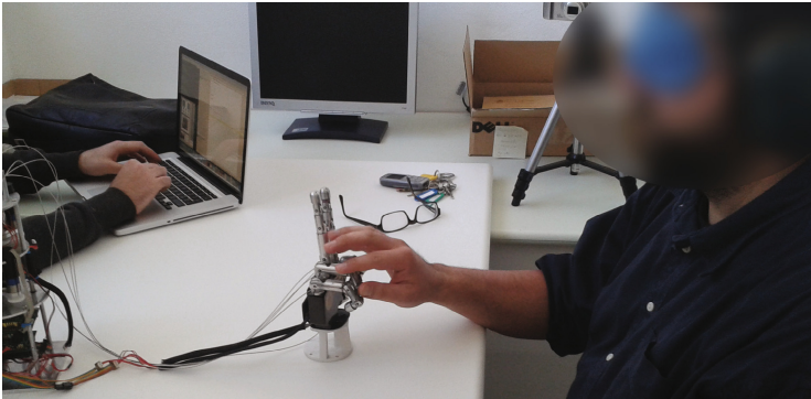
Fig. 9. Subject (blinded and with headphones) interacting with the robotic hand during the test session (V letter is performed in the picture)
