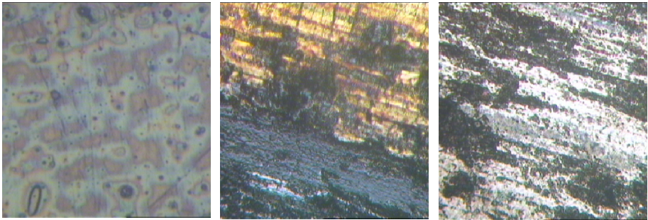
a. The surface morphology of friction pair before grinding
