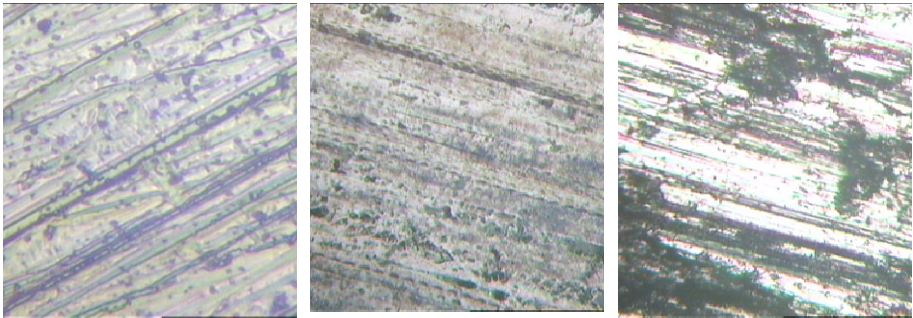
a. The surface morphology of friction pair before grinding b. The surface morphology of friction pair grinding 500 times c. The surface morphology of friction pair grinding 1000 times
