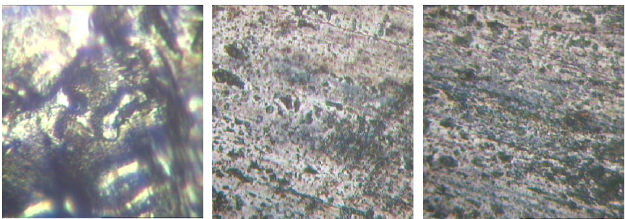
a. The surface morphology of friction pair before grinding
