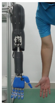
Fig. 1. A comparison between the IRR prosthetic arm-hand system and a male limb
