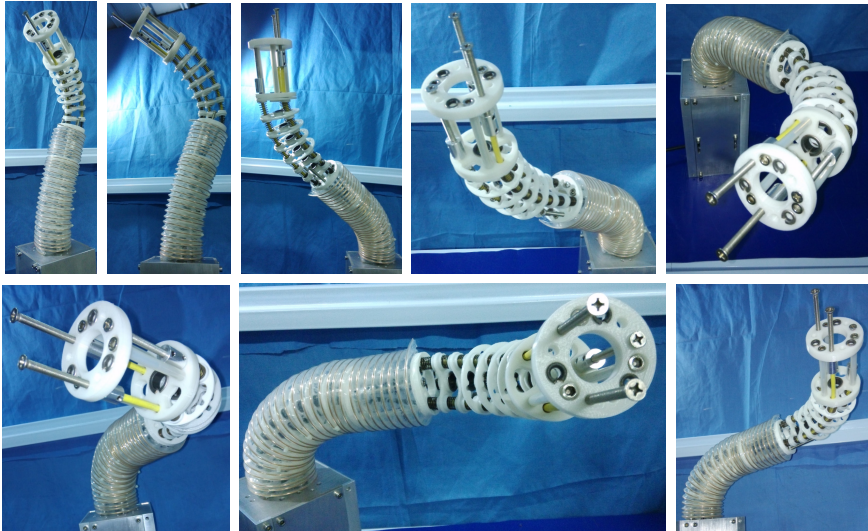
Fig. 6. ET Arm and its bending experiments
