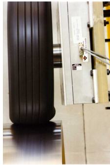
Fig. 4. Vertical stiffness test of a tire
