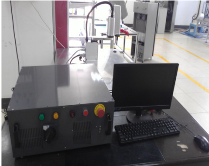
Fig. 7. The robot and its control cabinet
