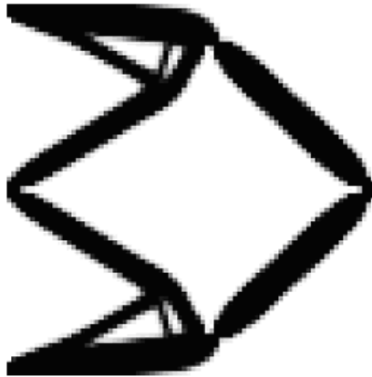
Fig. 5. Optimal mechanism obtained by the variable density method with filter technique
