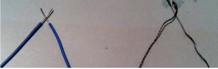
Fig. 3. Crossover contact points of copper wire lines and conductive thread lines
