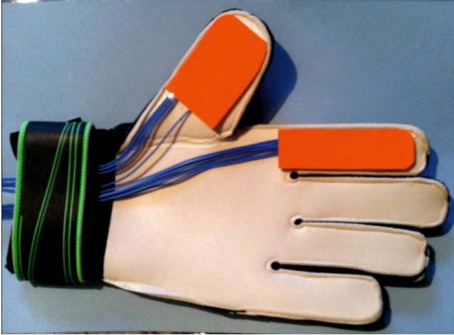
Fig. 8. Example of sensor attachment solution using a latex palm glove
