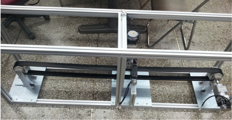
Fig. 7. 1/40 size miniature model of real flying touch hot rolling system for simulation
