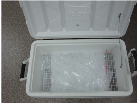
Fig. 4 Transport by insulated cooler with conventional ice cubes in Ziploc bags
