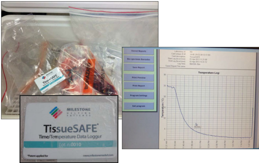
Fig. 5 RFID card records the run temperature
