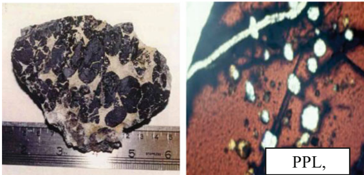
Fig. 14 (Second two, right ): (a) Nodular form of chromitite showing a grape-shot structure, where the rounded massive chromitite nodules are surrounded by dunite (SE Dhadnah area). (b) Photo micrograph of chromite grain under plan-polarized light showing the ordinary red-brown color of chromite with few silicate inclusions
