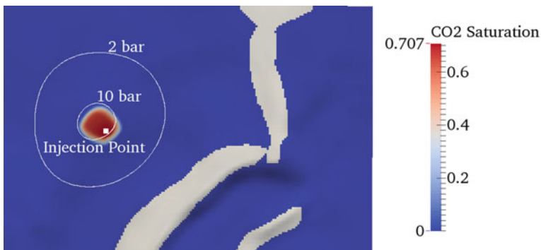
Fig. 9 Top view of the target formation (Solling) showing the CO 2 saturation at the end of the injection period (50 years) as well as two iso-lines of pressure increase. The grey area depicts the salt wall. The injection rate is 0.5 Mt per year
