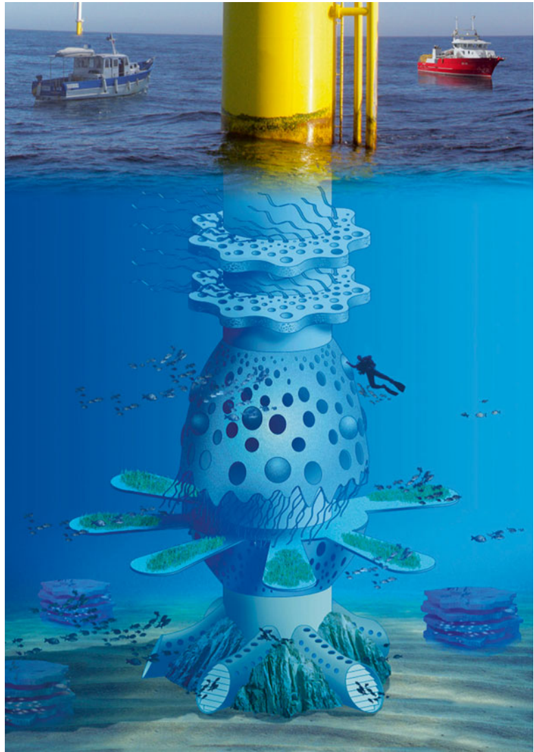
Fig. 5 Eco-designed offshore windmill foundation for fisheries enhancement and renewable energy production (in Lacroix and Pioch 2011)
