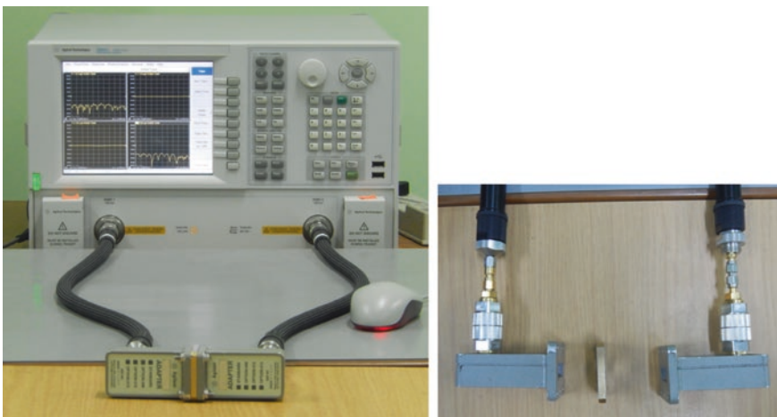
Fig. 1 A waveguide-based measurement setup using VNA. (Right) Components before assembly
