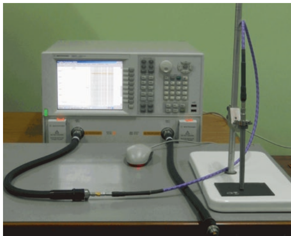
Fig. 2 Measurement of material properties using a VNA and open-ended coaxial line probe
