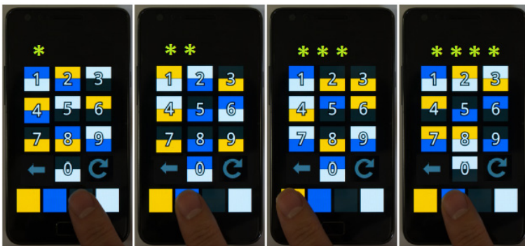
Fig. 4. Above figure shows user response for PIN digit 6. Each time user keypad gets partitioned using four colors. User needs to identify one of the correct color of his/her corresponding PIN digit.
