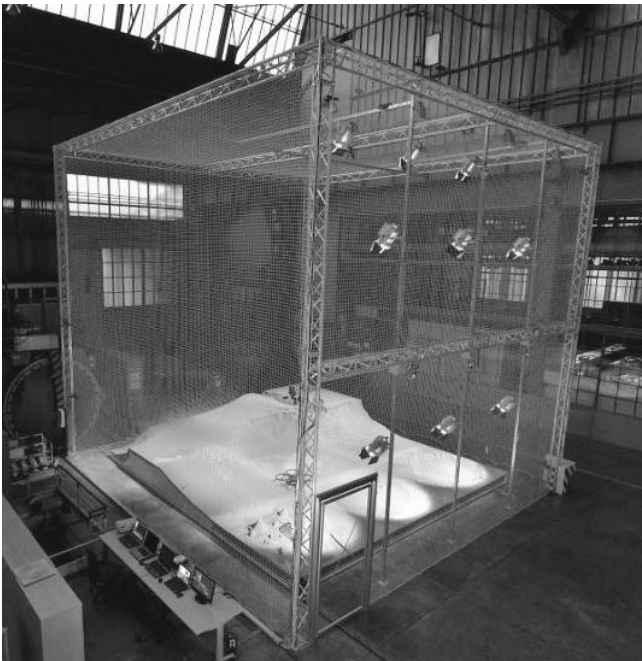
Fig. 2. The Vision-based Terrain Navigation Facility
