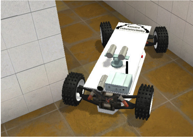
Fig. 3. Virtual mobile robot with 2 stereovision cameras and one rear camera
