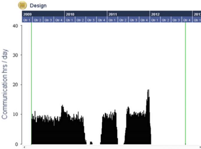
Fig. 8.9 The figure shows communication as forecast for the Design team, a subset of the total activity shown in the figure above. The demand for communication is driven by dependencies, meetings, and other factors. Still, the design team has limited capacity to respond, or perhaps other priorities. Very often, not all communication demand is satisfied, which can have delay and quality consequences
